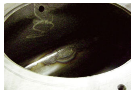
Figure 1 and 2: Roots pump seized by switching to ultimate pressure and the resulting local overheating
