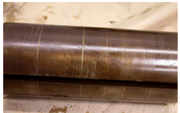
Figure 3 and Figure 4: Inlet port of a rotary vane pump without a dust filter. Rotor was tarnished in the cylinder. Pump system must be replaced.
