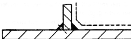
Figure 1: Double fillet weld (Source: Jobst H. Kerspe et al., Vakuumtechnik in der industriellen Praxis, expert-Verlag) [Vacuum technology in industrial practice]. The vacuum side is indicated by the dashed line.
