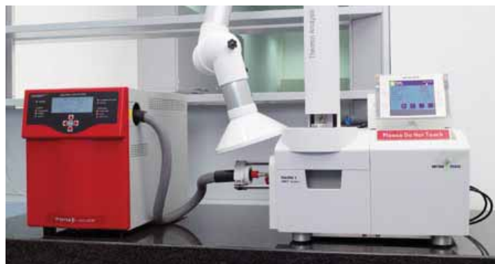
Coupling of a Mettler Toledo TGA/DSC 1 with a Pfeiffer Vacuum ThermoStar GSD 320
